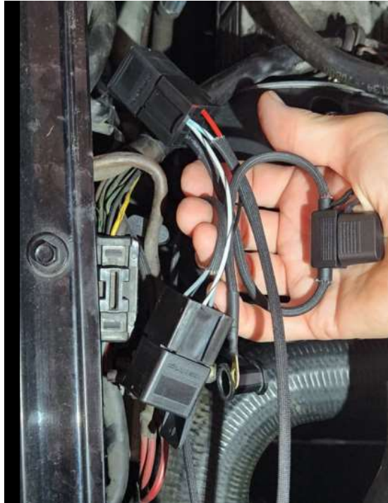
Relay Kit shown in installation area at front under-hood side near jump post
