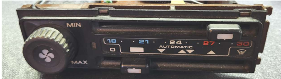
1980 – 1995 928 AC Controller Head A/C Compressor activation relay is internal
