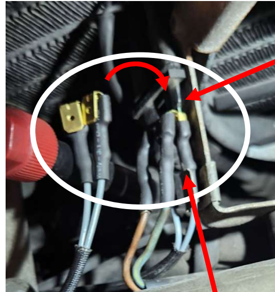
Piggyback wires attached above freon temp switch above receiver/drier. No polarity.
