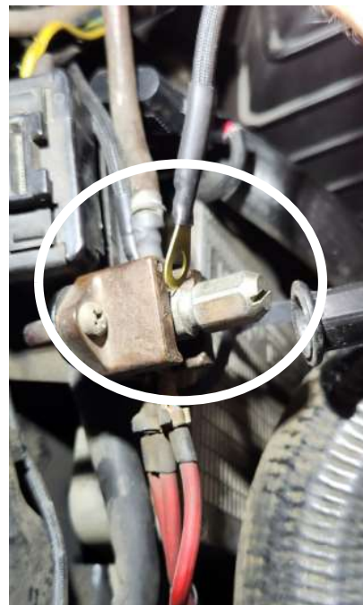
Piggyback wires attached above freon temp switch above receiver/drier. No polarity.
