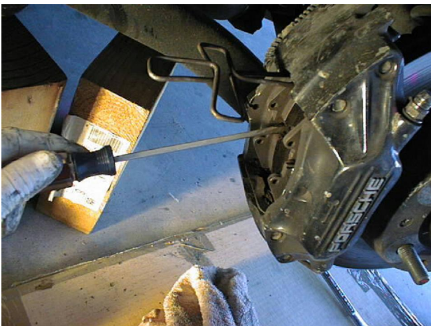
the front calipers are held on by 2 rather large allen bolts. You may need a cheater to aid in loosening the bolts.
