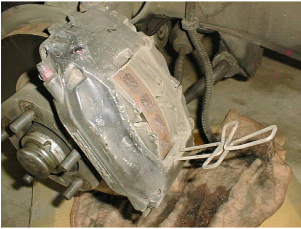
front brake retaining spring removed to access pads
